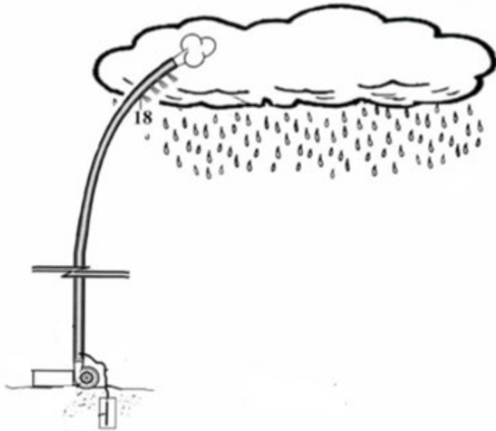
Figure 2 illustrates a cloud seeding system using hoses.
