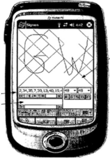
Handwriting input using a grid defined on the screen of a mobile phone.
