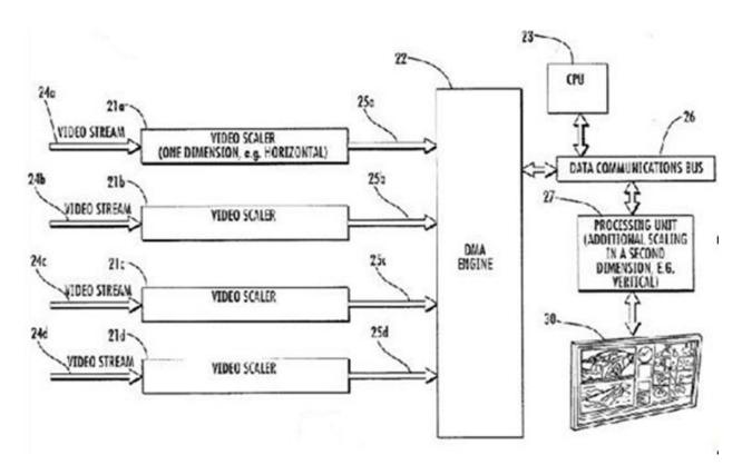
In the figure above, the processing unit is coupled downstream from video cross-point switcher for generating additionally scaled video streams by additional video scaling on initially scaled video stream.
